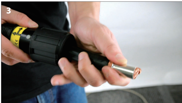
Strip back the cable jacket by around 33mm, then slide on the reduction sleeve over the exposed conductor strand.
