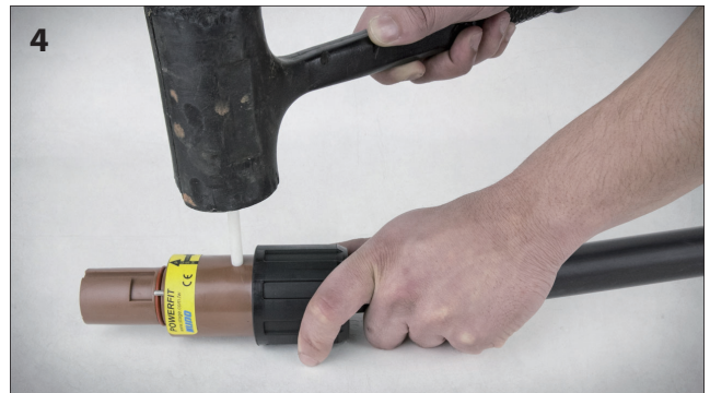
When inserting the cotter pin into the insulator, it is easier to hammer it in from the chamfered side of the cotter pin.
