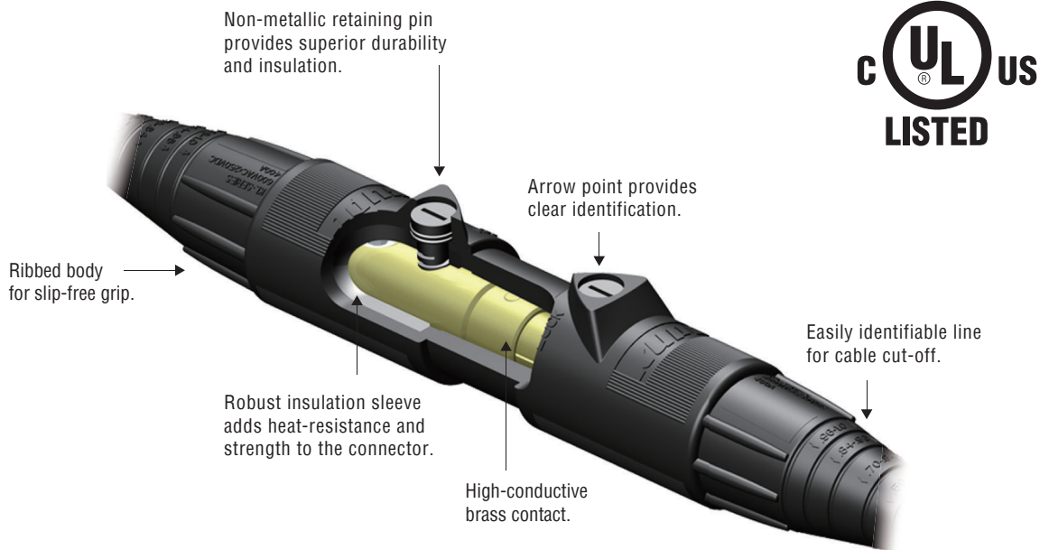
Wide range cable access form 0.33" to 1"
