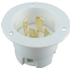
ATL-1530FI Locking Flange Inlet Pin: 4 / AMP: 30 / Voltage: 250 NEMA: L15-30
