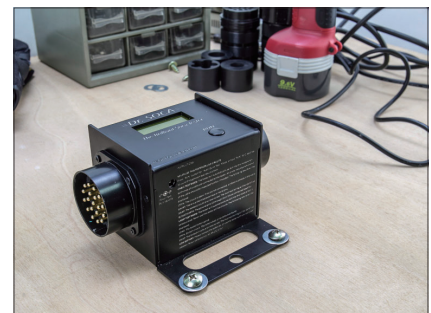
Bolted to a work bench without movement for better cable testing job.
