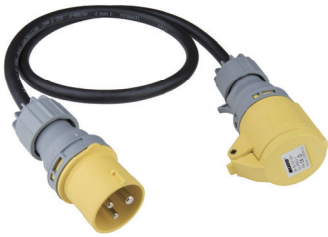
Cable: H07RN-F 3 x 2.5mmsq Connector: 16A 2P+E CEE form (110V)
