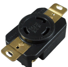
ATL-630R Locking Receptacle Pin: 3 / AMP: 30 / Voltage: 250 NEMA: L6-30R
