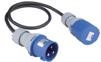
Cable: H07RN-F 3 x 4.0mmsq Connector: 32A 2P+E CEE form (230V)
