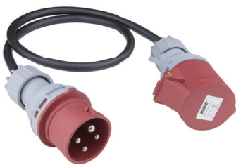
Cable: H07RN-F 5 x 2.5mmsq, or PVC 4C x 14AWG Connector: 16A 3P+E CEE form (380V)
