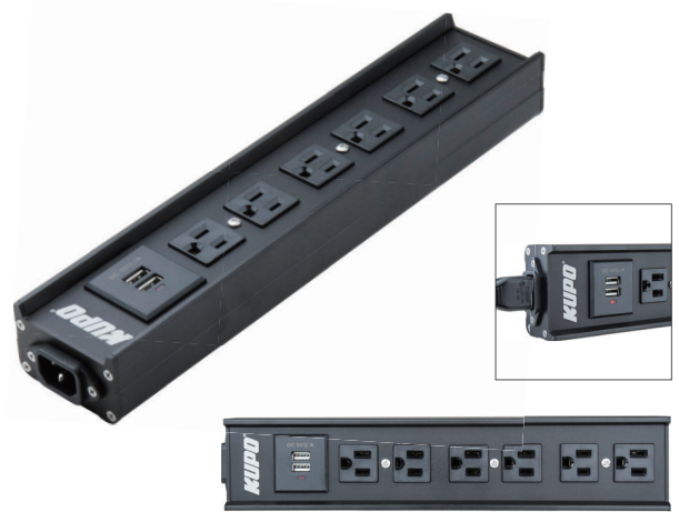
PDB-L1604 6 Way Linear Distribution Box with USB Charger Input: 1 x 10A IEC male socket Output: 6 x NEMA 5-15 Edison outlets Dimension: 326(L) x 66(W) mm x 42(H)/mm
