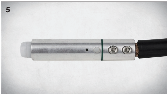
Slide the cable with reduction sleeve into the contact, then use a 5mm a/f allen key to tighten both set screws. 10.5N/meter (min. required)
