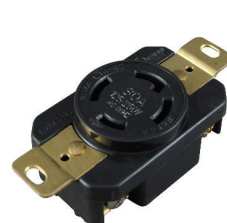
ATL-1430R Locking Receptacle Pin: 4 / AMP: 30 / Voltage: 125 / 250 NEMA: L14-30R
