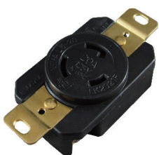
ATL-520R Locking Receptacle Pin: 3 / AMP: 20 / Voltage: 125 NEMA: L5-20R
