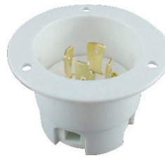
ATL-1520FI Locking Flange Inlet Pin: 4 / AMP: 20 / Voltage: 250 NEMA: L15-20
